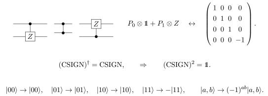
The csign also has an essentially classical truth table. The AND or the inputs is placed in the phase bit.
